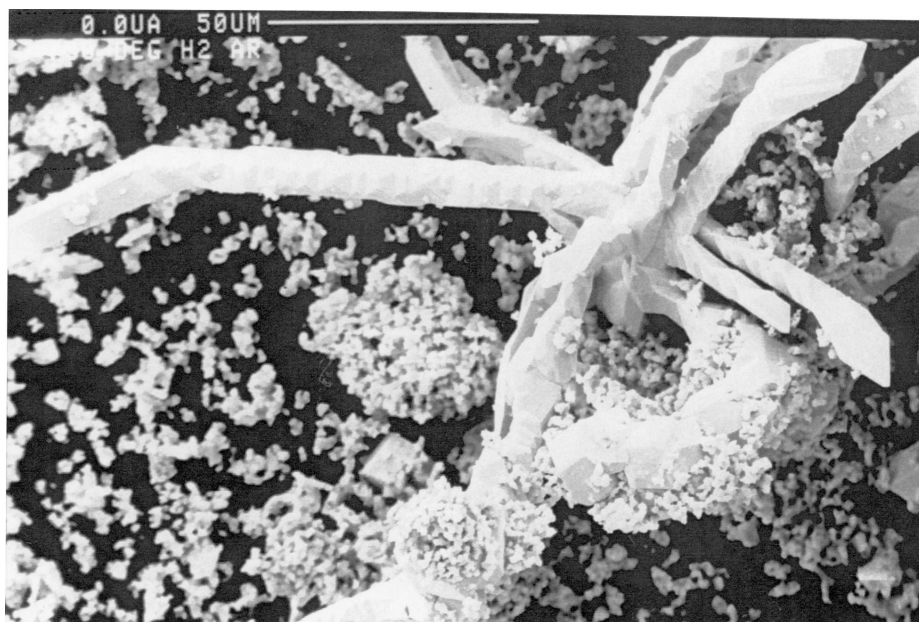
Figure 10 Presence of a large tungsten trichite for a high humidity condition.
